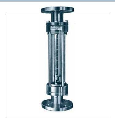
The direct reading flowmeters of the FD series have a rigid support structure consisting of 4 C/steel columns. The connections to the process can be threaded or flanged. The measuring tube is made of boron-silicate glass which is perfectly calibrated and therefore easily replaced by the user without needing to change the float. It is sealed with adjustable gaskets and glands.
