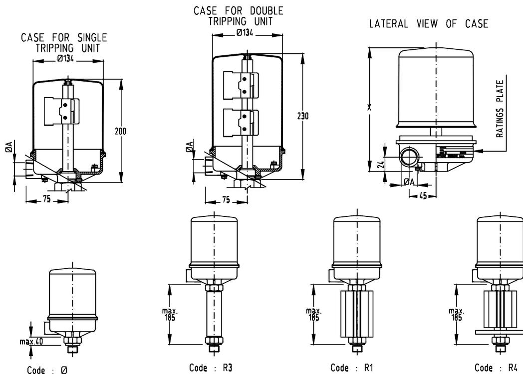
SPACE NEEDED FOR REMOVING THE CASE COVER: X = 320 (CASE WITH SINGLE TRIPPING UNIT)
