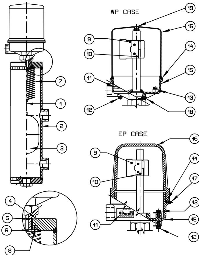
When ordering spare parts, always indicate the instrument's serial number. You can find it on the ratings plate on the case (see Pos. 11) and has 5 digits preceded by the letter "F" (e.g.: F45678).
