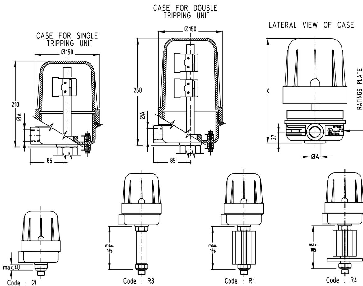
SPACE NEEDED FOR REMOVING THE CASE COVER: X =340      CASE WITH SINGLE TRIPPING UNIT
