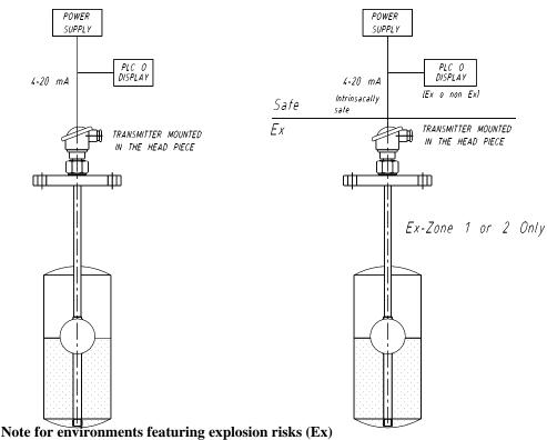
The level transmitter shall operate through an Eexi-certified barrier for zones 1 or 2.
