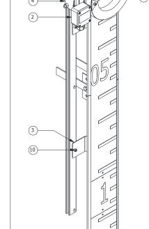
Mount the two brackets (3) on the scale's guide by passing two screws (12) through the bracket and trough the two holes on the back of the scale's guide.
