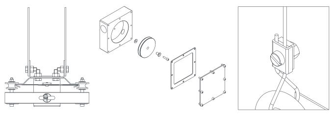
Place the index (10) in front of the graduated scale by sliding it from the top with the scale's guides between the index's wheels and connect the index (10) to one end of the external wire (16) with the clamp (2).
