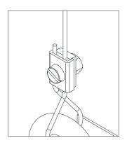
Place the Guide Index (10) in front of the graduated scale making it slide from the top with the graduated' scale guides between the index's rollers, then connect the index (10) to one end of the rope (11) with the clamp (2) Disassemble the covers of the  $90^{\circ}$  return idlers (26).
