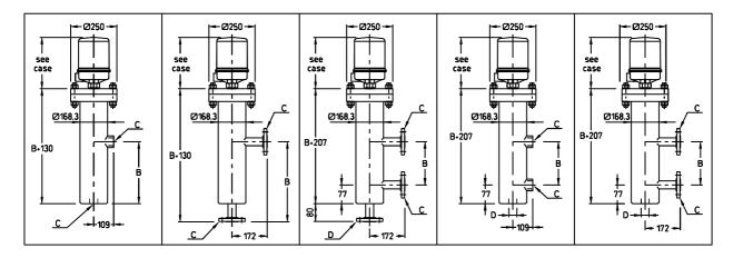
Dimensions to order  $\mathbf{B} = \text{field } \mathbf{C} = \text{connections } \mathbf{D} = \text{draining}$
